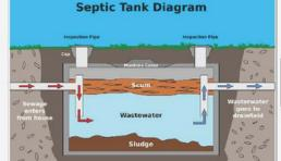
Modern septic tanks have two compartments, but the idea is the same the effluent is seen here labeled as wastewater'
