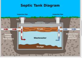
Modern septic tanks have two compartments, but the idea is the same the effluent is seen here labeled as 'wastewater'
